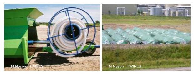
In the EcoPOD© system, a hydraulic ram pushes material from a feed-hopper into LDPE bags. A 60 m bag holds 100 m3 of wastes aerated by perforated pipe connected to a fan.
